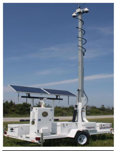
The BroadView 2 Video Camera Trailer from American Signal Company is a multi-functional necessity to complete your work zone or security application. The PTZ dome camera and communications system can monitor traffic for volume/occupancy/speed and relay data to an ITS work zone system, and provide crucial intelligence for incident management. Utilize onboard storage while also streaming your feeds. The BroadView 2 is suitable for any environment needing a highly portable platform.
