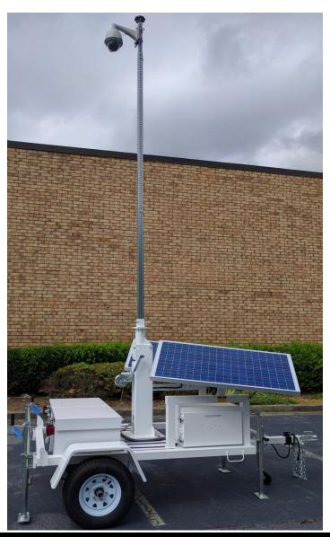
The BroadView 1 Video Camera Trailer from American Signal Company is a multi-functional necessity to complete your work zone or security application. The PTZ dome camera and communications system can monitor traffic for volume/occupancy/speed and relay data to an ITS work zone system, and provide crucial intelligence for incident management. Utilize onboard storage while also streaming your feeds. The BroadView 1 is suitable for any environment needing a highly portable platform.
